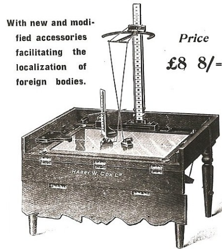
Figure 7. The [Sir James] Mackenzie Davidson [1857-1919] cross-thread localiser was based on the principle of triangulation and was the most popular of several techniques for determining the position, including depth below the skin surface, of foreign bodies such as pieces of shrapnel or bullets. It was developed in 1897 and was the first method to use mathematics for the localisation process. [29-31] Full description of the theory is given by Walsh. [32]
